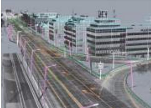
The Hardbrücke road bridge in Zurich was mapped very quickly, including surroundings, using mobile terra® systems, generating data for planning and restructuring.
